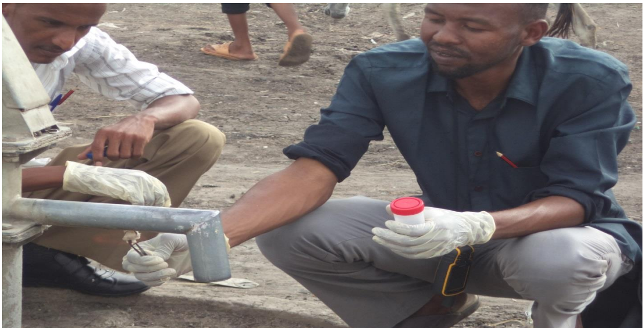
Disinfection for Sampling from Han-Pump
