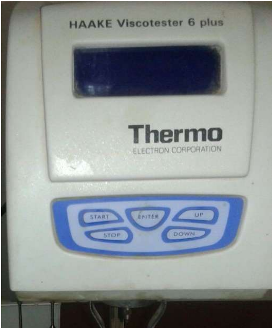
Figure (5-1). Viscometer to measure oil viscosity
