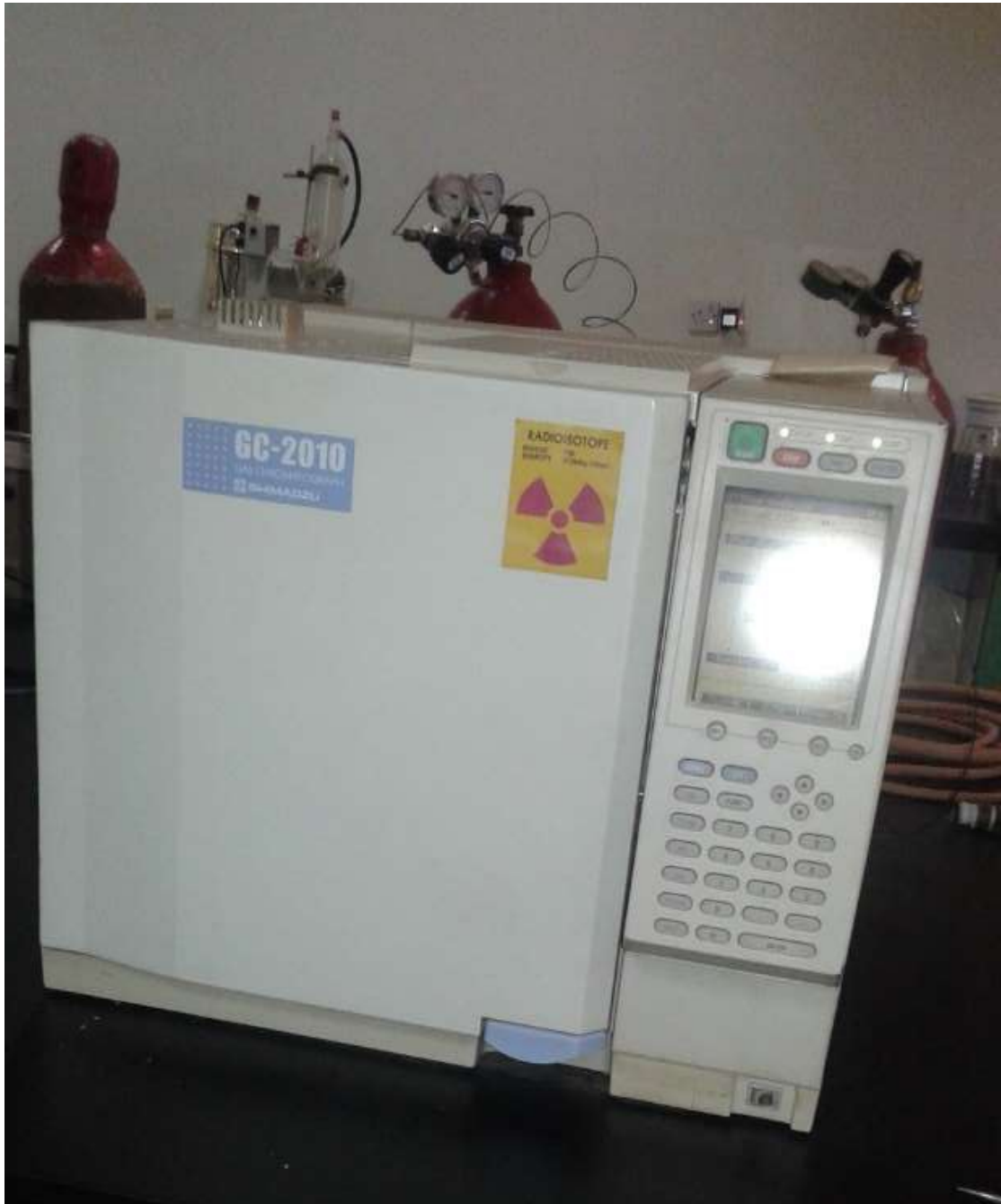
Figure (5-2). GC-MS system to detect the compounds in essential oil
