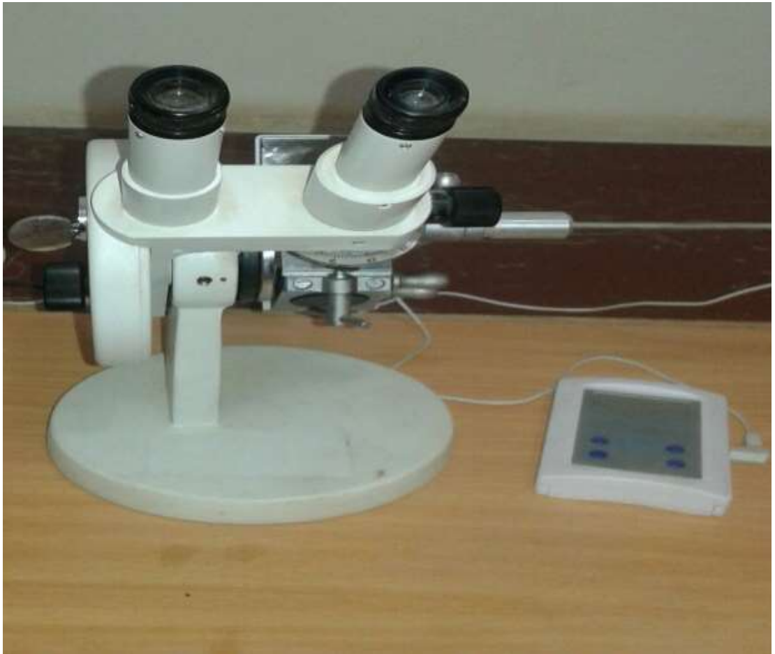
Figure (5-4). Refractometer to determine refractive index of oil
