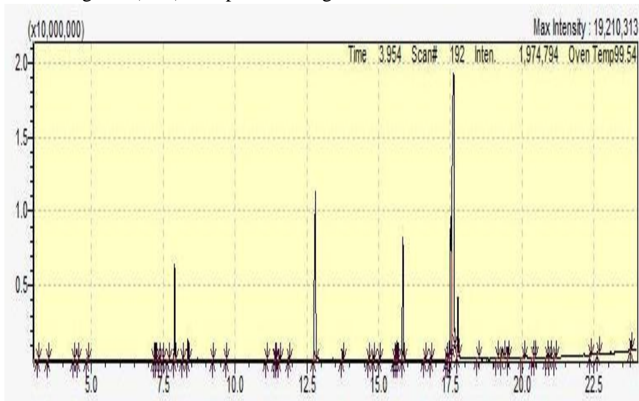
Fig.3.44. Typical total ion chromatogram
